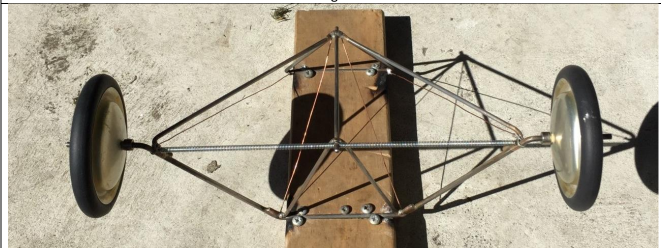
Under carriage experiment with spring loading by Norm Rogers Photo Henny Remkes.
